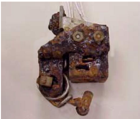
Untreated - failure after 100 hours saltspray test
